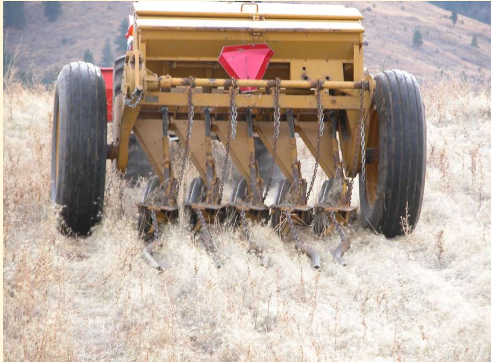
Photo 4. Drill seeding controls seeding rates and promotes germination by placing seeds at specific depths.
