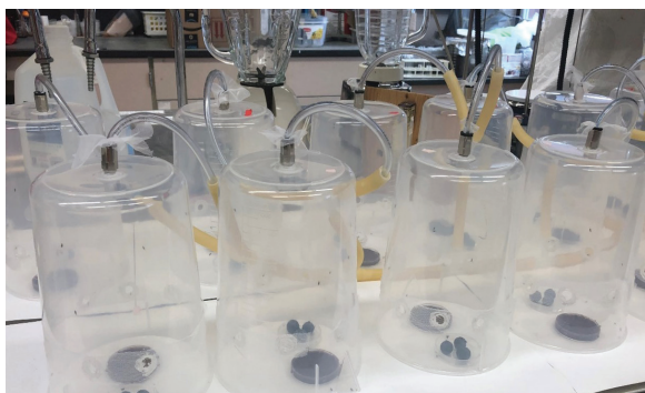
Figure 1. The experimental setup of the laboratory trials. Ventilated arenas were constructed from plastic beakers that contained ventilation holes and a plastic tube connected to a vacuum pump to ensure airflow (Tait et al. 2018). 12 adult Drosophila suzukii (6 males and 6 females) were released into each arena for a 24-hour period. Each arena contained 3 Pinot noir grapes and either 5 mL of water (control treatment) or 5 g of the arrestant. There were 10 replicates per each treatment per trial for all three trials.
