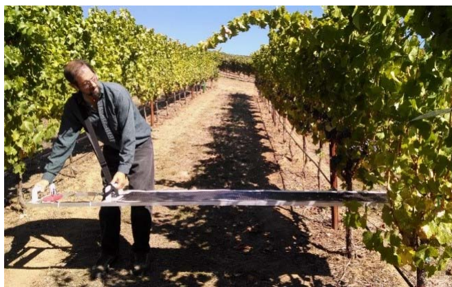
Figure 1. A Paso Panel can be constructed to measure the canopy shaded area for calculating the crop coefficient ( K_c ) for grapevines in the field. Measurements are taken at solar noon when the smallest shadow is cast by the canopy (not the case in this photo). (Photo by Vinay Pagay)
