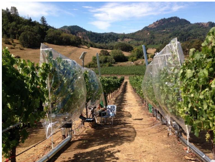
Figure 2. Whole-canopy chambers (“balloons”) used in a research block to measure the water use of fully-irrigated Tempranillo grapevines at Abacela Winery, Roseburg, Oregon. (Photo by Vinay Pagay)
